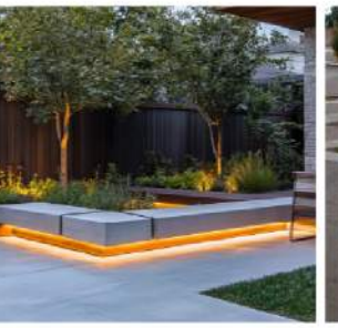
E BENCH TOEKICK LIGHT • FLEXIBLE LED CHANNEL AT TOE KICK OF CAST IN PLACE CONCRETE BENCHES
